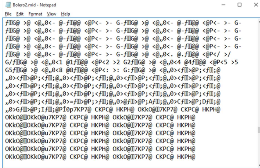
Figure 6.2: A window showing a segment of the Maurice Ravel's Bolero. Three different arrangements of character strings indicate different passages within the musical piece. The entire file is about 180 times larger than the segment shown here.
